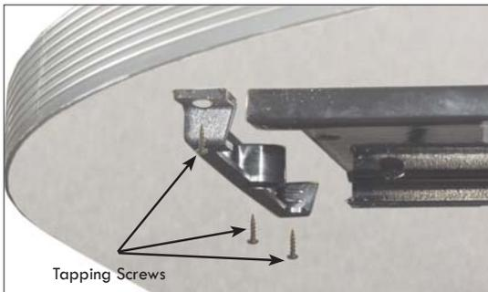
Place the track guard over the end of the track and attach in the center hole first using (1) #8 x 5/8" Round Head Philips Recess Type "A" Tapping Screw.
