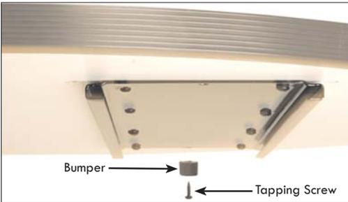
Push the screw thru the bumper and attach to the track. Make sure screws are tight enough to remove a slight bow from the track.
