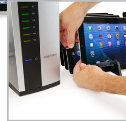
30-Pin or Lightning USB cables attach from each device to a designated slot on the back of the tower
