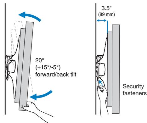
No knobs or levers are used to activate the tilt motion or hold the position of display!
