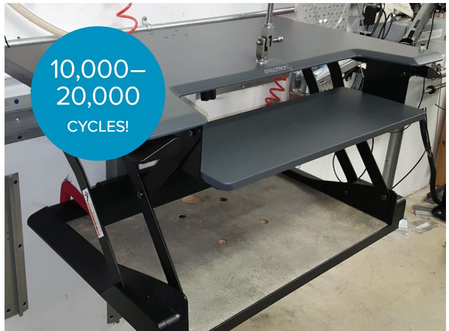
Cycle test for height adjustment
