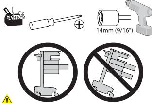
**CAUTION:** Close worksurface before opening drawers. Open only one drawer at a time. Do Not push cart when drawers or worksurface are open. Failure to follow these instructions may cause the cart to be unstable.
