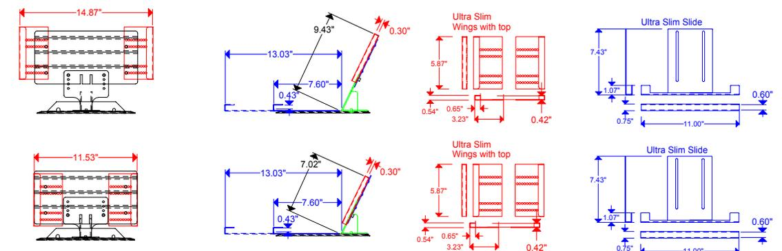
Wing screw head is .120" high, Slide screw & washer are .170" high
