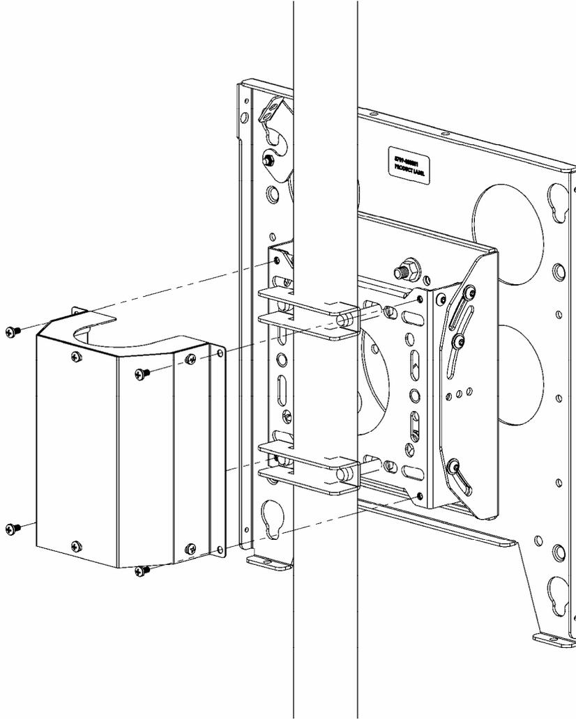
**Figure 3. TPA-105 on Pitch-Adjustable Mount**
