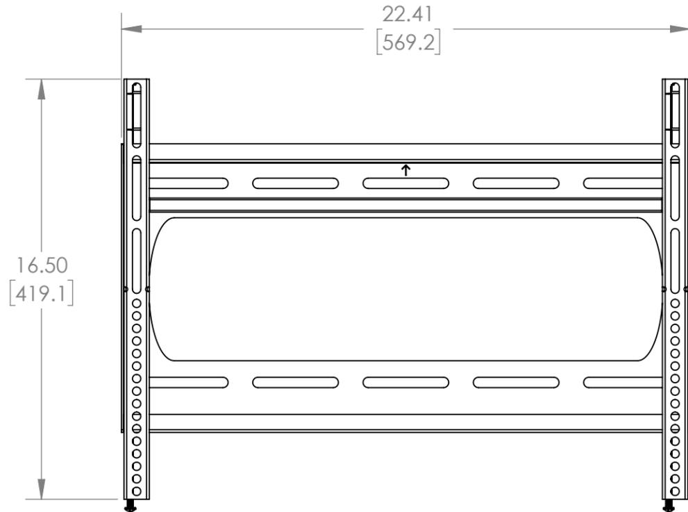
14 GA (.074") ASTM 1008 COLD ROLLED STEEL MATERIAL
