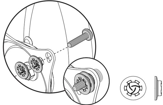
The Universal Spacers will fit M4, M5, M6 and M8 screw sizes.
