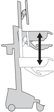
Once the camera has been mounted to the shelf, it is important that you adjust the lift tension for the additional weight. Test the lift tension by moving the head unit up and down. If it travels smoothly and easily through the full range of motion, and does not drift up or sag down from the place you set it, the tension is good. If not, adjust as directed below:
