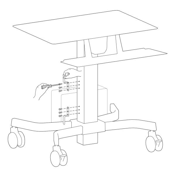
**16** NOTE: Leave enough slack in cable to allow full range of motion.
