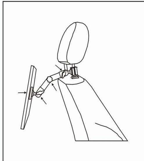
4. Screw the TRAY with ARM and adjust the knobs to make TRAY into perfect position.
