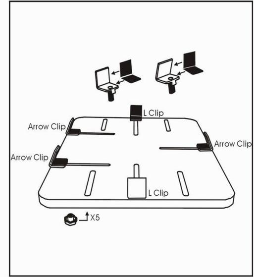
3. Stick the L CLIPS and ARROW CLIPS with PROTECT PADS and screw onto the TRAY with TRAY SCREWS.
