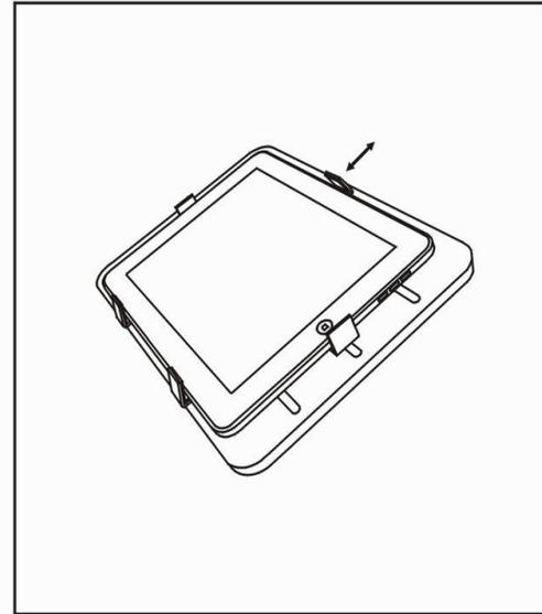
5. Only adjust the upper TRAY KNOB to put on or take out the ipad or the other elec device. The TRAY can be install on any tripod.
