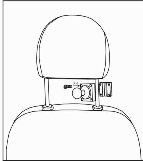
1. Screw the BASE A and BASE B on the headrest support with 4 BASE SCREWS.
