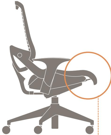
Pressure under the thighs is reduced by allowing the waterfall to act as a flexible suspension. This “lobster” mechanism engages the pin at seven positions via the molded detents. The waterfall is adjusted without a lever or knob by pushing the edge of the seat down.
