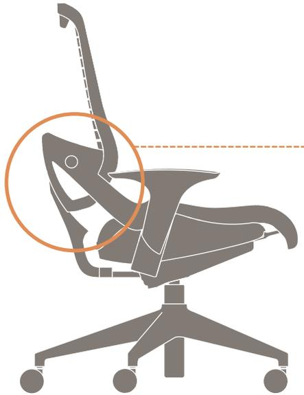
The user feels back support because the roller will not move unless the user shifts their weight to override the ramp. The ramp acts as a virtual lock; once overridden, the chair may recline. This mechanism eliminates the need for a lever or knob and prevents lock out.
