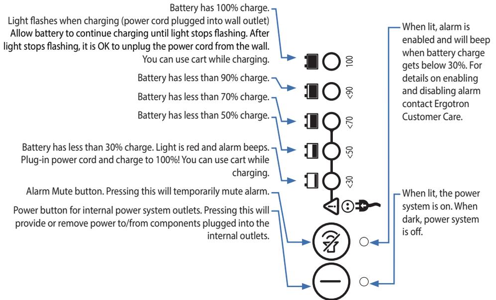
**NOTE:** Frequent operation of the cart while battery charge levels are below 30% will significantly reduce the life of your battery.
