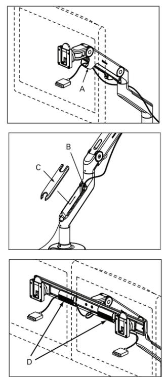
*Note: For dual-monitor applications, first route monitor cables through cable management clips (D), then refer to Step a.*
