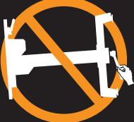
**Cart Must Remain Upright! Tipping Cart On Side May Cause the Work Surface to Disengage Causing Serious Personal Injury and Property Damage.**
