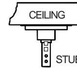
60mm long curved carriage bolt is used as a pin to attach extension column to stub. Center lock nut secures the assembly.
