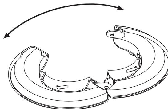
2 Wrap escutcheon ring (A) around extension column and snap into place to cover hole in ceiling tile.
