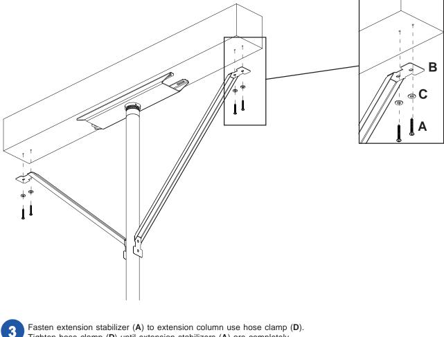
Fasten extension stabilizer (A) to extension column use hose clamp (D) Tighten hose clamp (D) until extension stabilizers (A) are completely secured and column is stabilized.
