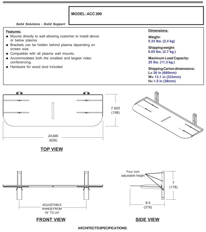
The plasma video conference shelf shall be a Peerless model ACC 309. It shall include all mounting hardware for attachment to wood studs. It shall have height range eight inches. It shall have the ability to mount on 16, 20 or 24 inch wood studs centers. The finish shall be a scratch resistant black fused epoxy. Assembly and installation shall be done according to instructions provided by the manufacturer.
