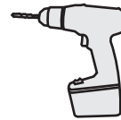
Drill with 1/8" (3mm) bit (Wood stud wall)
