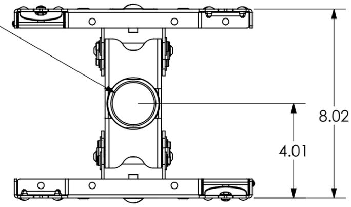
NOTE: CUSTOM INTERAFCE BRACKET NOT SHOWN. THE CUSTOM INTERFACE BRACKET NEEDED FOR YOUR DISPLAY WILL ADD BETWEEN 1/2" AND 2" IN DEPTH AND MAY AFFECT LOCATION OF DISPLAY ON THE MOUNT.
