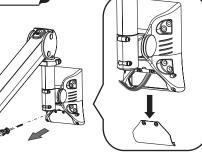
Fix the Monitor on the VESA mount using Allen Key and screws.
