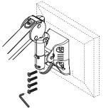
Please insert the cable to the monitor, complete the circuit and then fix the cap.
