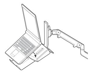
Attach the supplied squares of self-adhesive hook-and-loop tape to the underside of your dock in an evenly spaced straight line to ensure that squares are aligned with the hook-and-loop strip that is
