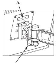
If desired, friction on the Ball Joint may be increased. This can be achieved by tightening the (3) Ball Joint Friction Screws (a).
