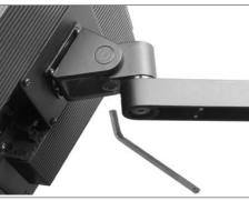
Tilt the monitor so it faces upward and locate the set screw under the tilter. Insert the 7/32" Allen wrench into set screw to adjust the tilt friction.
