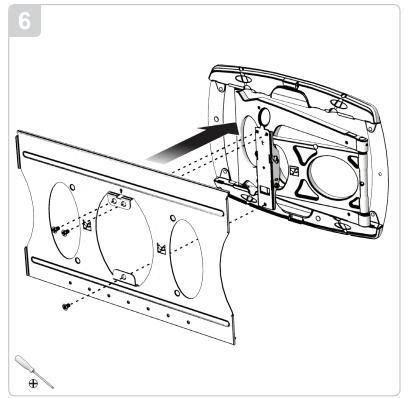
Re-install the front wall arm plate to the arm with the three M5 flat head screws you set aside earlier. Confirm screws are fully seated and tight.
