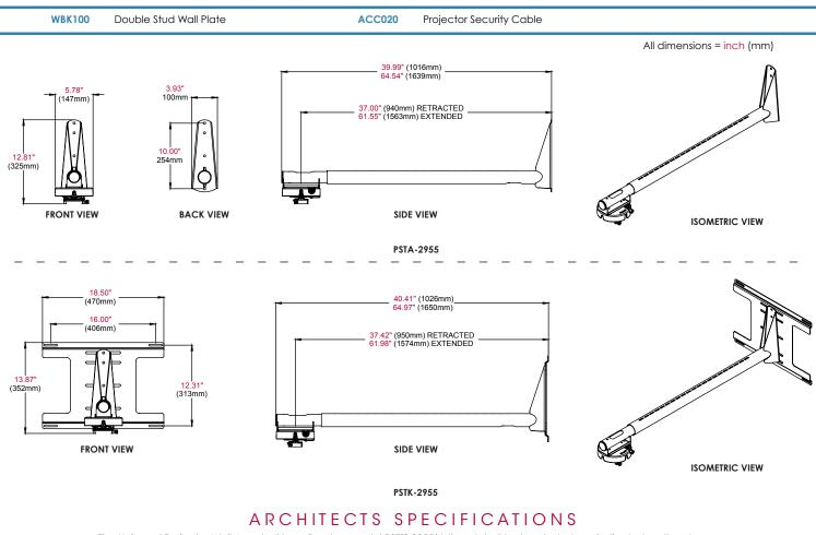
The Universal Projector Wall Arm shall be a Peerless model PST%-2955(-W) and shall be located where indicated on the plans. It shall be constructed of heavy gauge cold rolled steel and feature scratch resistant white and black fused epoxy finish. Assembly and installation shall be done according to instructions provided by the manufacturer.
