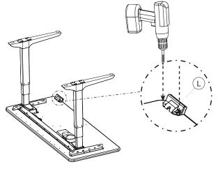
Attach Switch (L) to underside of tabletop using two smaller (#8 x %") Sheet Metal Screws (J) For Silhouette tops, use 2 Type 23 Screws (H).
