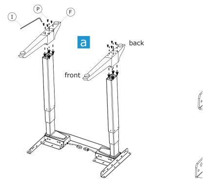
5 Attach Base to Tabletop and Tighten Screws
