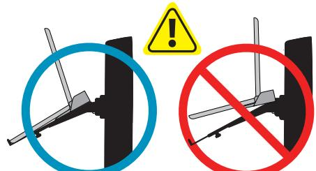
To ensure stability, the docking station SHOULD NOT extend over the back of the tray.
