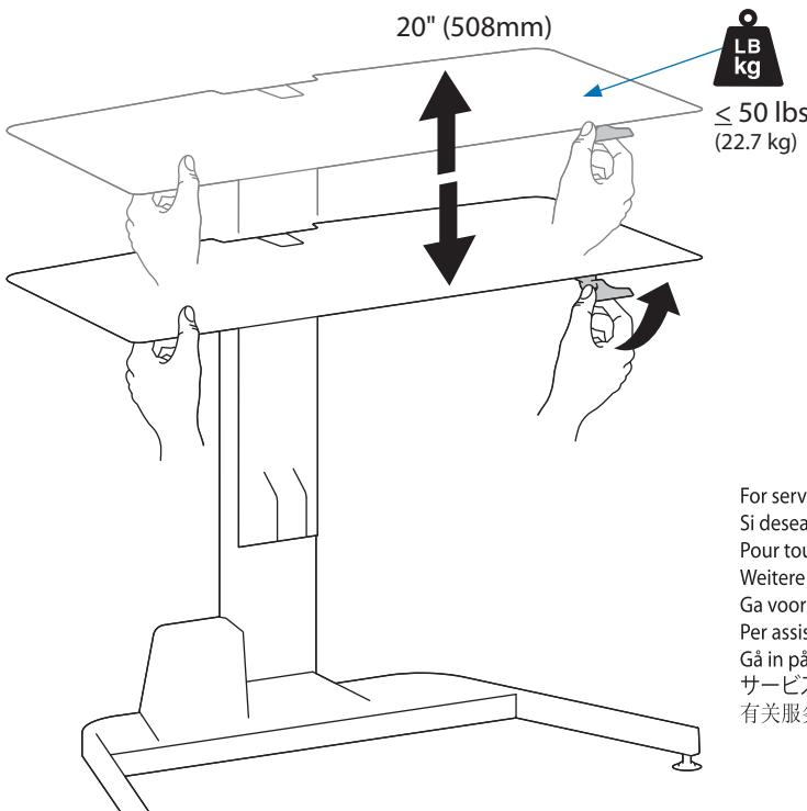
**WARNING!** The addition of accessories can negatively impact the tip performance.
