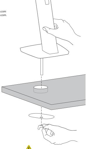
Caution: Bolt must be located in center of grommet hole.
