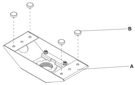
Use stud finder to locate stud centers. Use anti-vibration mount (A) as a template to mark slot centers on stud centers.
