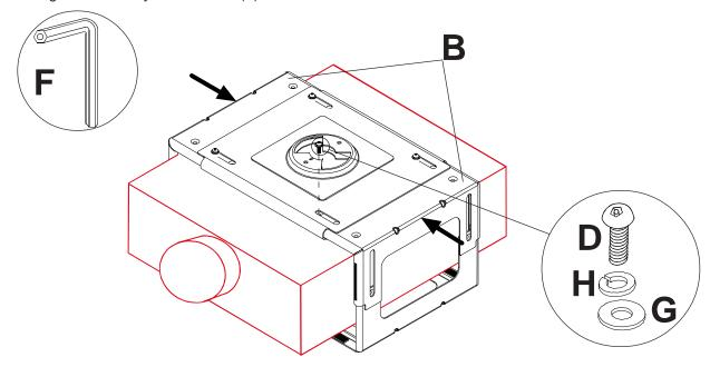
Slide top assembly downward until top and bottom sides are against projector (as shown). Fasten with four M6 screws (**D**), lock washers (**H**), and flat washers (**G**). Tighten using 4 mm security allen wrench (**F**).
