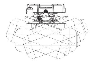
SWIVEL (YAW) 360° (when attached to an extension column), +/- 15° (when flush mounted)
