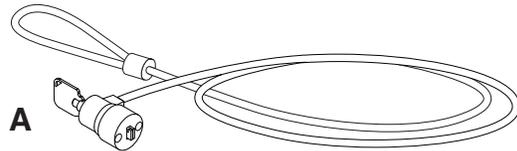
**1** Wrap cable assembly around extension column and insert lock mechanism through cable loop as shown.
