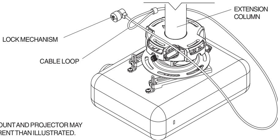
**2** Insert key into lock mechanism and set to open position by pushing in key and rotating until hooks are in open position as shown in figure 2.1.
