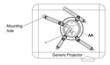
Attach adapter plate (AA) to projector using one screw (BB, CC, DD, or EE) for each channel as shown below. Tighten all screws, while keeping the center of gravity. Be sure that adapter plate (AA) is straight. Adjust the feet of the channels to keep the adapter plate level. Tighten all screws with 4 mm security allen wrench (FF) or wrench provided with projector mount, while keeping the center of gravity. If M3 screws are used, tighten using 2 mm security allen wrench (GG).
