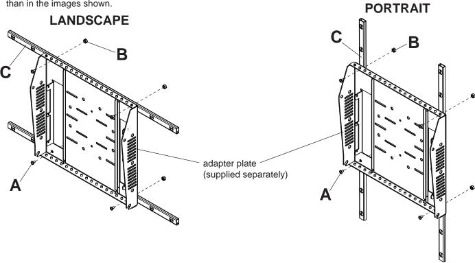
Attach adapter brackets (C) to back of screen using screws and washers provided with your model.
