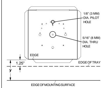
**Note:** To figure out where to mount swivel base so TV is flush with the edge of the mounting surface, use the following formula:
