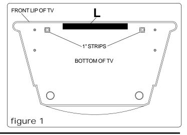
1-1 Turn TV upside down and determine mounting locations. For TV's with a flat front, make sure that leading edge of screen is flush with leading edge of tray. For TV's with a curved front, mount screen as close to the front of leading edge of tray with tray still being hidden. Attach tray to TV by installing four screws (**B**) into TV mounting bosses.
