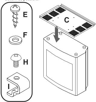
Slide upper tray (C) back until fully engaged. Firmly hold in position while you insert and tighten lock plug (G), several turns, until fully engaged.
