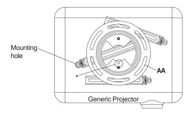
Attach adapter plate (AA) to projector using one screw (BB, CC, DD, or EE) for each channel as shown below. Tighten all screws, while keeping the center of gravity. Be sure that adapter plate (AA) is straight. Adjust the feet of the channels to keep the adapter plate level. Tighten all screws with 4 mm security allen wrench (FF) or wrench provided with projector mount, while keeping the center of gravity. If M3 screws are used, tighten using 2 mm security allen wrench (GG).
