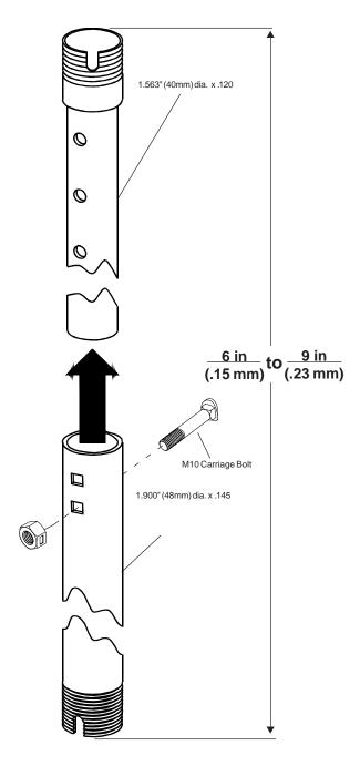
The "tube in tube" design of the Adjustable Extension Column allows it to be adjusted, within its specified range, at 1 inch (25 mm) increments. The bolt and lock nut provided securely locks the two tubes together at the desired length.
