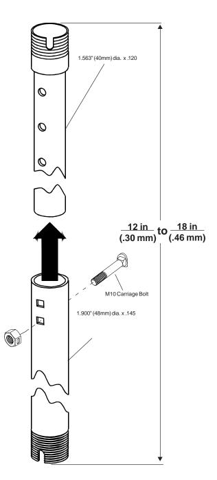
The "tube in tube" design of the Adjustable Extension Column allows it to be adjusted, within its specified range, at 1 inch (25 mm) increments. The bolt and lock nut provided securely locks the two tubes together at the desired length.
