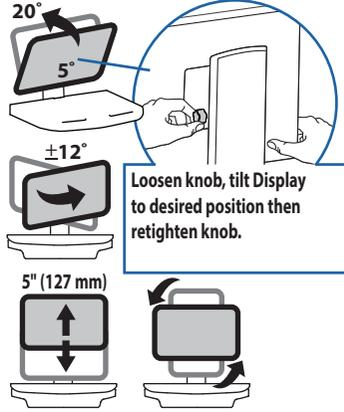
Loosen knob, tilt Display to desired position then retighten knob.
