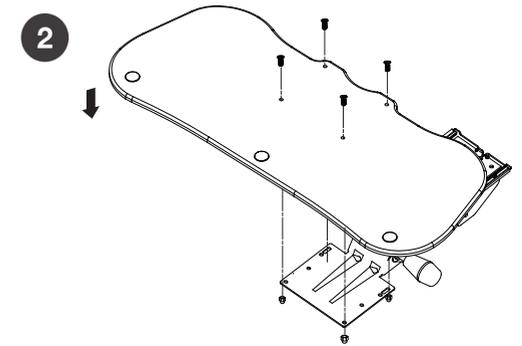
**Second**, line up the screw holes on the keyboard tray **platform** with the holes on the keyboard mechanism. Line up and insert the 4 **M5x17** screws into the indicated holes on top of the keyboard tray platform and line up and place the 4 **M5 acorn nuts** to the underside of the mechanism. Once in this position, screw in and tighten the M5x17 screws into the M5 acorn nuts.
