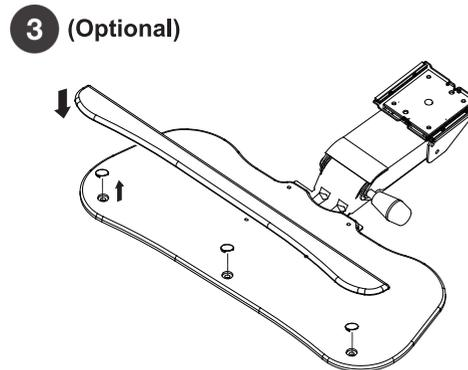
Remove the 3 caps on the end of the keyboard tray and place in a safe location. Attach the wrist rest until you feel all 3 placements have been magnetically secured.
