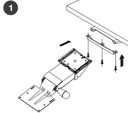
**First**, slide the keyboard tray **mechanism** onto the tracks on the underside of the EasyLift Desk.
