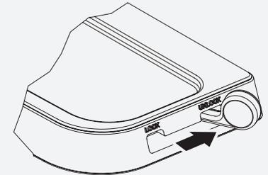
Slide lever into unlock position.
