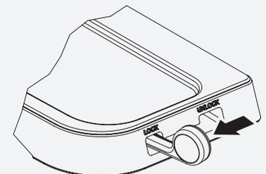
Slide lever into lock position for maximum stability.
