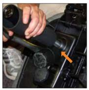
Firmly holding the cylinder with one hand, use hammer to strike the mechanism around the cylinder entry point.\*\* Several strong blows may be required to dislodge the cylinder from the mechanism.
