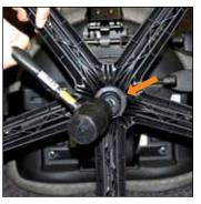
Using a plastic hammer, strike the bottom of the cylinder while firmly holding one leg of the base to dislodge the base from the cylinder.\*
