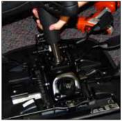
Slip cover over the top of new cylinder and then insert into the mechanism.
