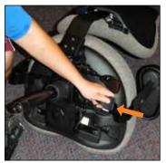
Extend cylinder to full length using seat height lever. Slide cylinder cover fully away from the chair so its out of the way.
