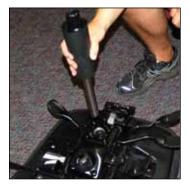
With cylinder out of the mechanism, slide the cover off. You may reinstall the old cover on new cylinder, or use new cover (Step 6).
