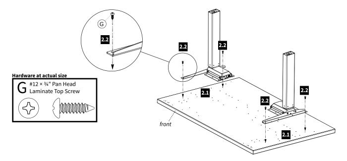
**2.3** With frame set positioned and the four corner screws secure, attach frame set using the remaining  $#12 \times 3/4$ " Pan Head Laminate Top Screws (G).
