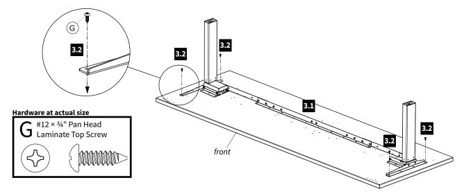
**3.3** With frame set positioned and the four corner screws secure, attach frame set using the remaining  $#12 \times 34$ " Pan Head Laminate Top Screws (G).
