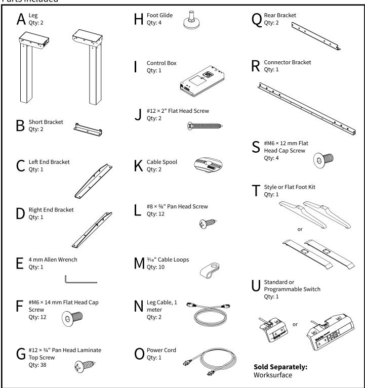
WARNING: Maximum loading of table assembly is 225 lb. (102 kg.). Maximum load includes the weight of the table top itself, any equipment placed upon it, and any equipment suspended or hanging under it. Loading should be evenly distributed over table surfaces. "Payload Capacity" is the Workrite Ergonomics recommended maximum loading which includes the Workrite sourced worksurface.
