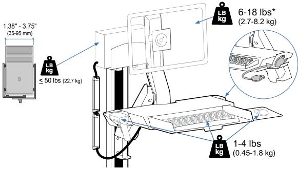
\* The Combo Arm can be modified to mount displays up to 20 lbs (9.1 kg), however display lift and tilt motion will not be possible if this option is chosen. Refer to special instructions on page 13.
