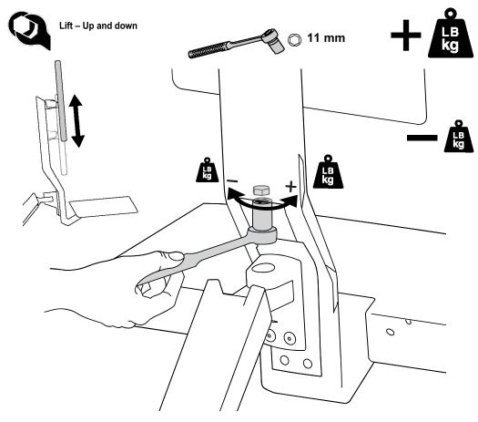
Increase Lift Strength If the mounted weight is too heavy or this product does not stay up when raised, then you'll need to increase Lift Strength:
