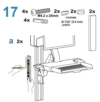
CAUTION: Make sure there is enough clearance between back of mounted component and cable channel. Failure to allow clearance space may result in personal injury and equipment damage.
